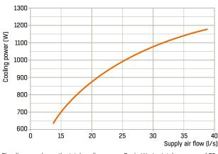
The diagram shows the total cooling power P<sub>tot</sub> in W at a total pressure of 70 Pa and a water flow  $q_w = 0.05$  l/s. Temperature difference between room air and supply air  $\Delta t = 8$  °C and the temperature difference between mean water temperature and room temperature,  $\Delta t_w = 8$  °C.
